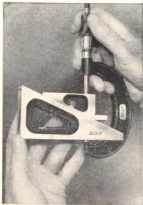
Gage Being Set to Micrometer Accuracy
